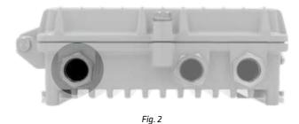
**3.** Tighten the connectors into the housing in accordance with the connector manufacturer's specification. The recommended torque force for the PG-11-5/8 adapter ring is 15-16 Nm and 11-13 Nm for the coaxial connectors.
