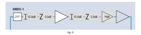
To prevent overdriving the RF amplifier, select 10 dB for the pre and interstage attenuator and EQ settings to 0 dB (*Fig. 11*).
